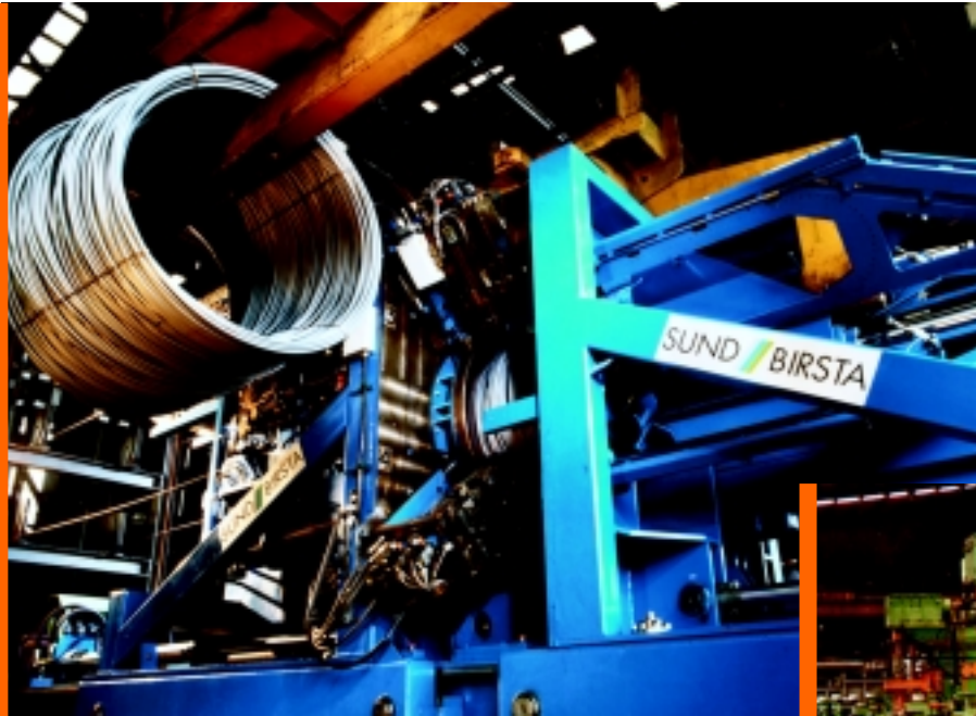
Wire rod packing machine at Amsteel Mills. Mesin menggulung rod wayar di Amsteel Mills.
