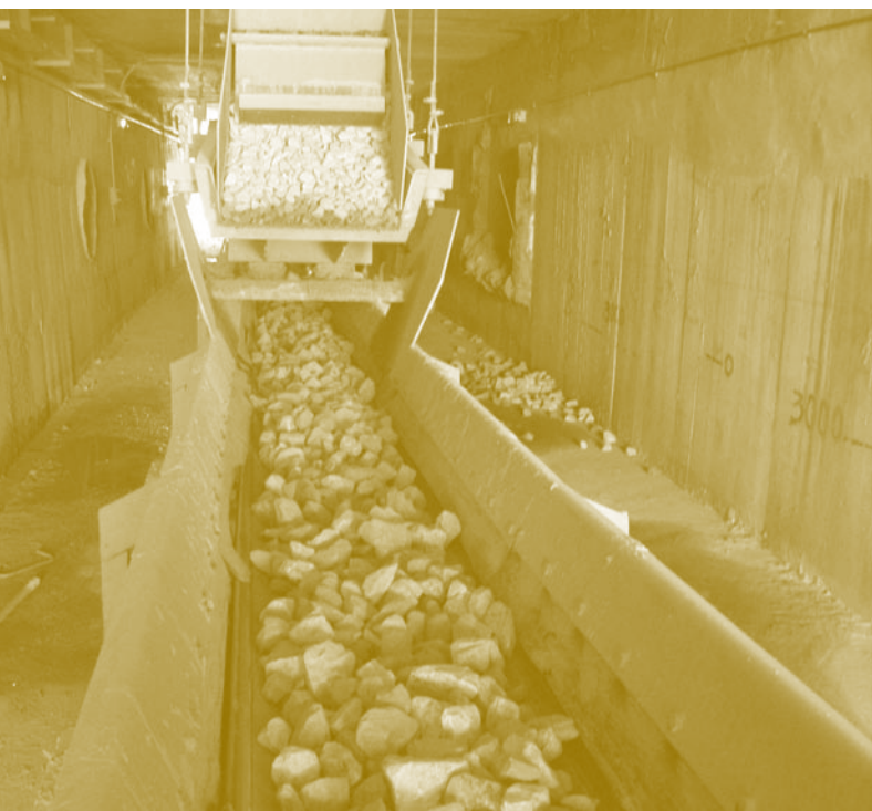
Limestone transferred by tunnel conveyor
