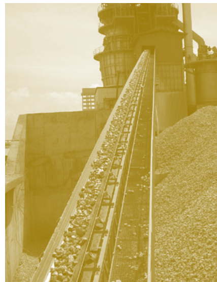
Limestone conveyed to intermediate bunker
